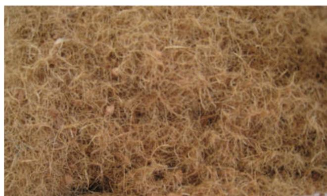
Figure 1. Dried Coconut husks and short Coconut coir fiber
