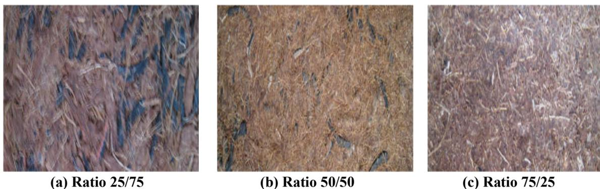
**Figure 6. Composite samples with different ratio of CCF/WTC**
