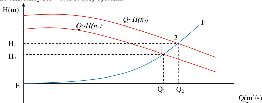
Figure 1. Characteristics of pump when rotation number changes
