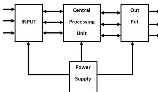
**Figure 4. Structure diagram of Programable Logic Controller PLC S7-200**
