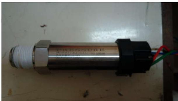
Figure 5. Pressure sensor RJ-131
