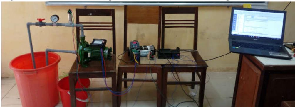
Figure 9. Automation system controlling pump head and discharge
