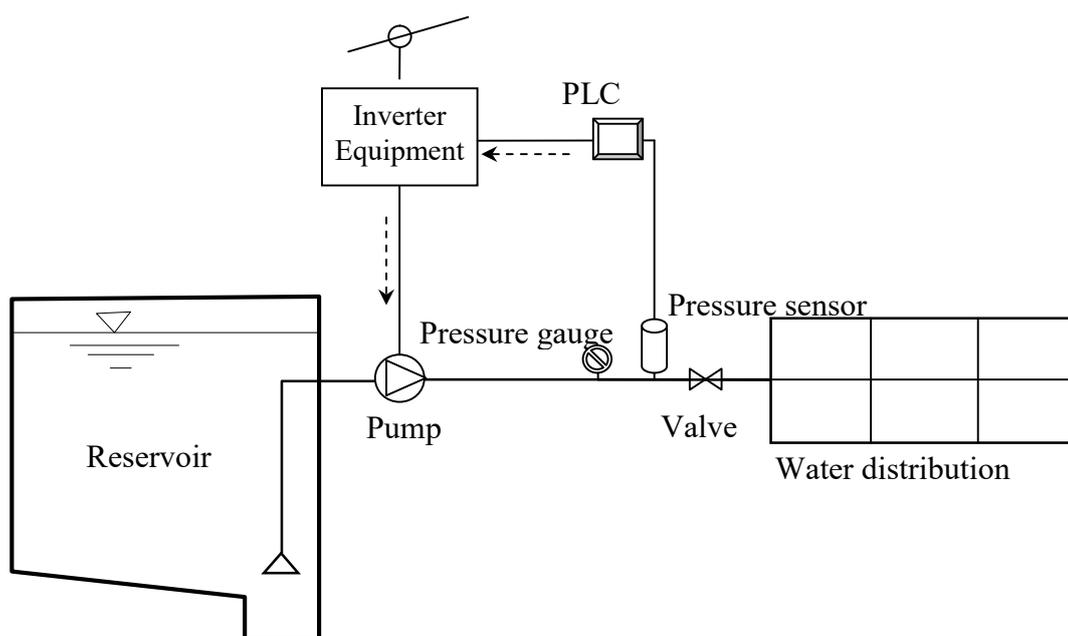
Figure 8. Diagram of a water supply system with automatic head and discharge control system
