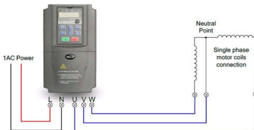
**Figure 3. Scheme for connecting MICNO-KE300 inverter with single phase motor**
