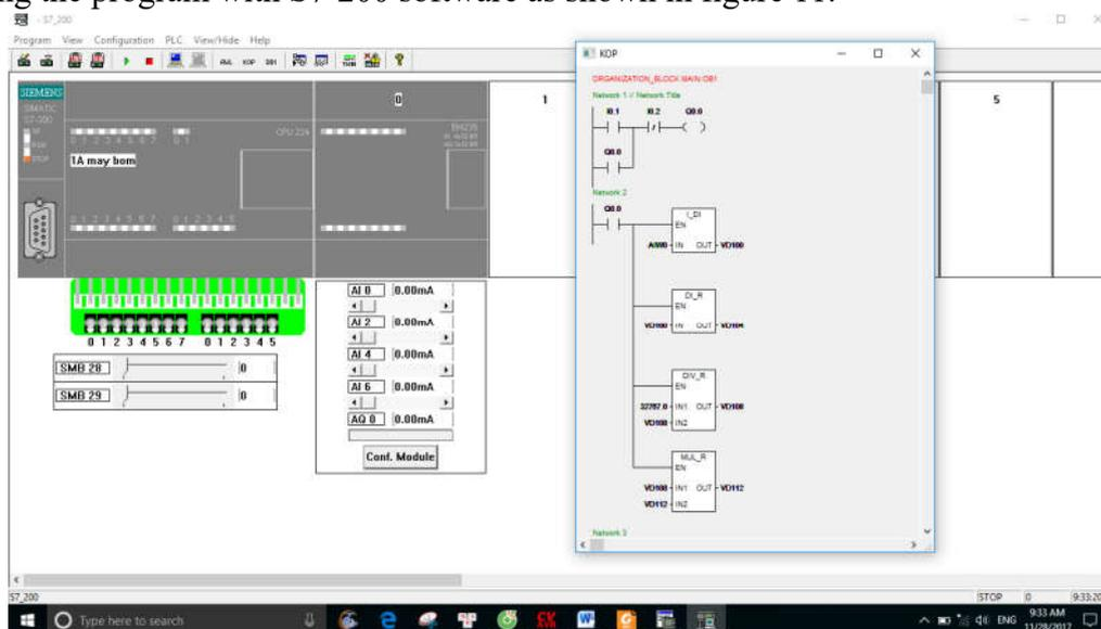
Figure 11. Running the program on Step 7 MicroWIN software
